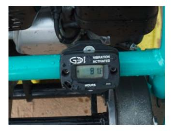
HOUR METER The plates can be fitted with hour meters to help monitor maintenance needs.
